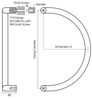
Dimension A 250mm C/C = 165mm curve 350mm C/C = 215mm curve
