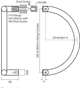
Dimension A 400mm C/C = 183mm curve 300mm C/C = 132mm curve
