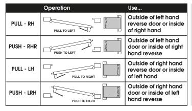
Please note: A left hand push paddle can be used as a right hand pull paddle: or a right hand push paddle can be used for a left hand pull paddle by turning over and reversing the paddle from its original mounted position. However, it is prefera-
