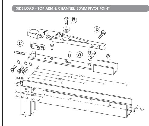
Prepare the top rail of the door as detailed, ensuring that the internal faces of the stile and top rail have been cut away to enable the closer spindle to be engaged during door hanging.
