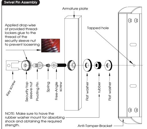
To assure a solid locking from the magnet and its armature plate, you need to mount the latter with FLEXIBILITY with help from the rubber washer supplied. A over tighten central screw or not enough power supply are the two main reasons why a magnet will not work with efficiency.
