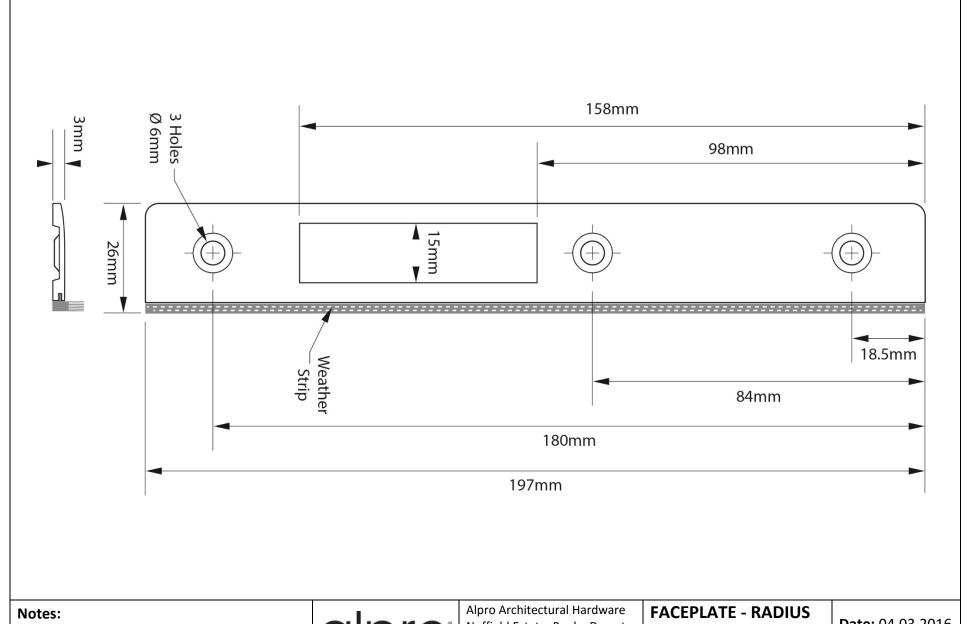
This drawing is not to scale. For use with Lock Type 52220 Finish SAA
