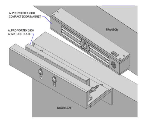
Installed magnet and bracket
